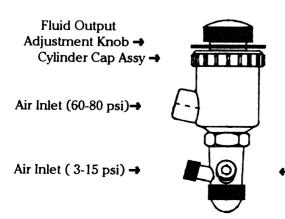
Air flowing back into the reservoir indicates the needle packing is worn and should be replaced. At this point it is recommended that an ES-370 Repair Kit, consisting of a packing assembly, needle, leather cup, air cap and tip be used to rebuild the spray gun.
